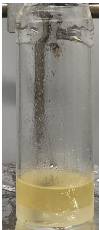
Figure 6.3. Glass reactor containing the reaction mixture of furfural hydrogenation by the in situ system ligand [Ir( \eta^4 -COD)Cl] 2 /6c. Reaction depicted: Table 6.1 Entry 11
